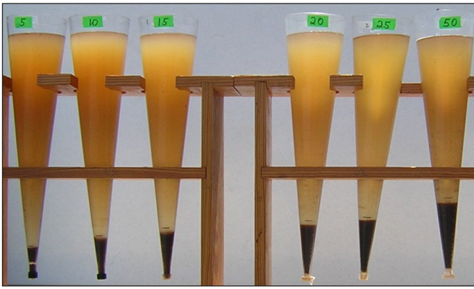
Figure 3. Imhoff cones to measure biofloc as the concentration of solids that settle after 10 to 20 minutes. The desired range for operation of biofloc systems is a settleable solids concentration of 10 to 15 mL/L for shrimp and 25 to 50 mL/L for tilapia.
